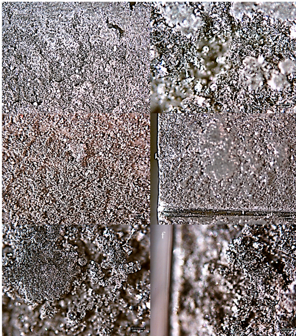
Figure 31. Adhesive 2 lap shear failure surfaces at different extension rates (a) 4× magnification at 25 mm/min; (b) 10× magnification at 25 mm/min; (c,d) 4× magnification at 500 mm/min; (e,f) 10× magnification at 500 mm/min.
