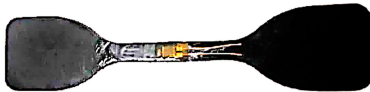
Figure 8. Tensile specimen with strain gage attached.
